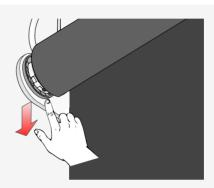
4.2.7 **Press and hold** the ■ stop button for 6 seconds.
